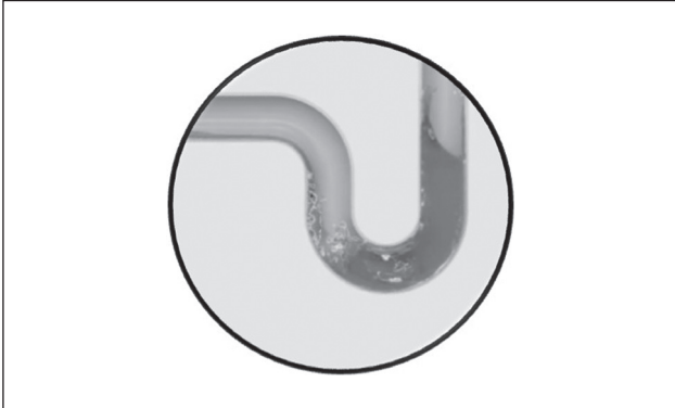
Figure 3. Trap seal breach
